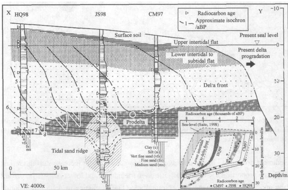
Fig. 2. Stratigraphy of a longitudinal cross section (X-Y) and accumulation curve for each borehole site and a late Quaternary sea-level curve for the East China Sea. Isochron lines are based on  $^{14}\text{C}$  dates and accumulation curves (modified after Hori et al.).
